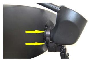
5 - While sitting in the passenger seat, place the mount over the mirror stem. Tighten the CLAMP SCREW until the mount starts to clamp onto the mirror stem. Position the mount as far forward as it will go and paralell to the bottom of the mirror before fully tightening.
