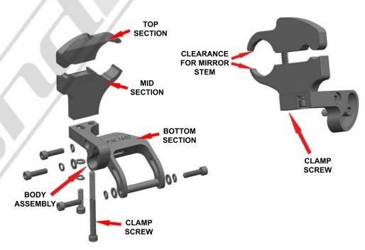
4 - The Body Assembly must be removed to gain access to the CLAMP SCREW. Remove the two socket head screws as shown above. Be sure to remove the lock washer with the top screw along with the lock washer and flat washer with the bottom screw. Loosen the Clamp Screw so there is enough clearance between the TOP and MID SECTIONS to slide over the mirror stem.
